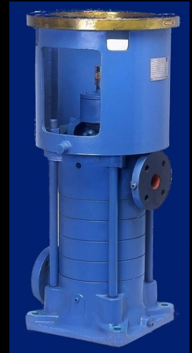
Vertical Multistage Pumps RKB Delivery size up to 250 mm Capacity up to 750 m 3 /hr. Head up to 580 metres
