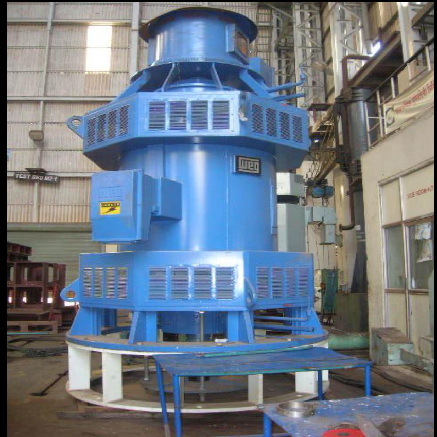
4mw Electric Motor For Testing Of Primary Sodium Pump
