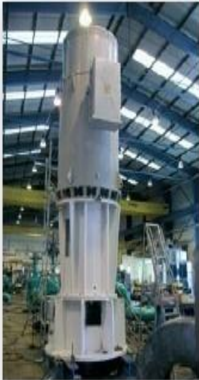
SPP vertical lineshaft pump directly driven by a 1200kw electric motor
